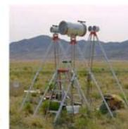
Figure 4: Scintillometers
